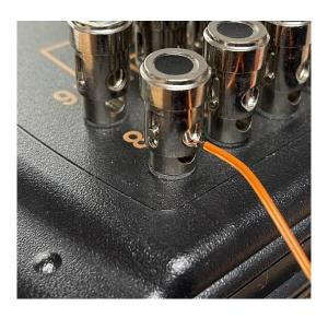
STEP 1: From the above picture, press down on the cue terminal. Insert one of the igniter wires. Release the terminal – spring force will clamp the wire.
